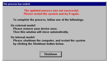
Remove the USB Card Reader, or click the Shutdown button, and reboot PC. After removing all memory cards, retry the update (Refer to "2.2. Updating process").
