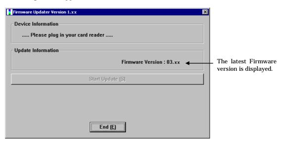
5) When the USB Card Reader is recognized, the current firmware version is displayed and the Start Update [S] button becomes enabled.
