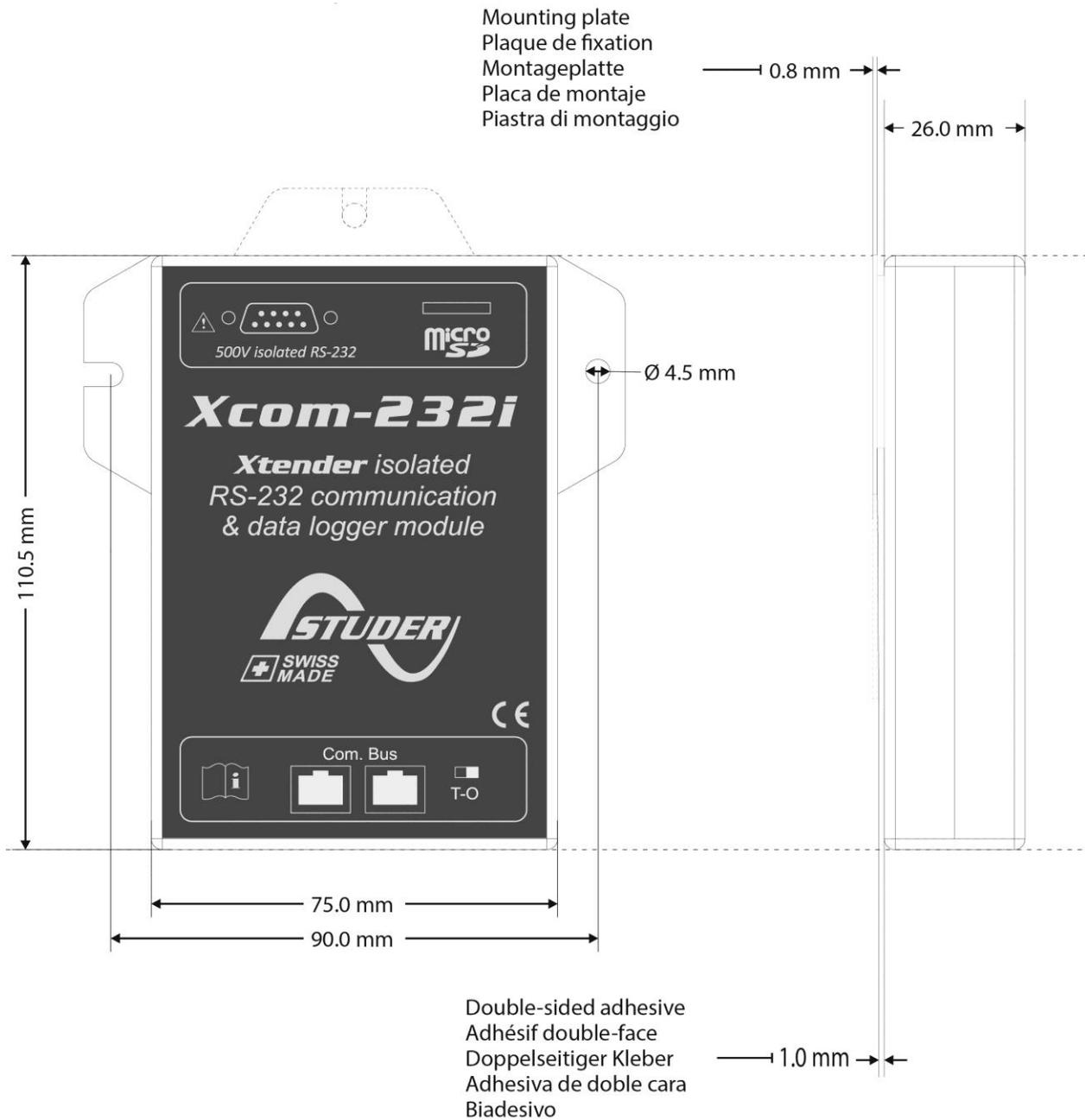
Figure 8: Views of different sides with dimensions
