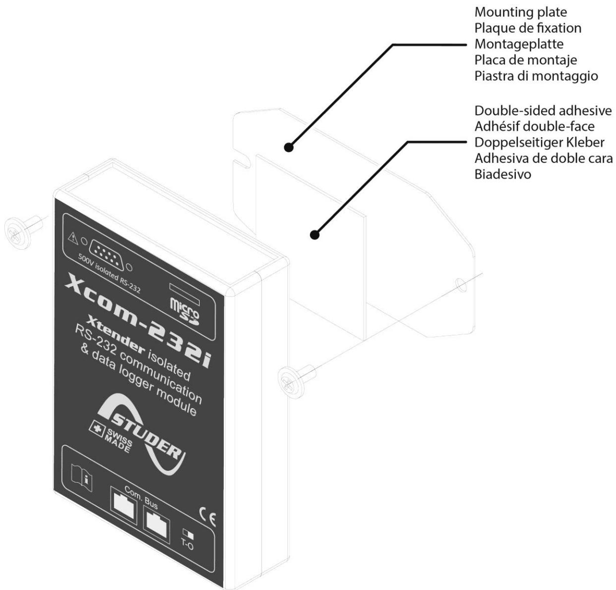
Figure 9: Mounting of the Xcom-232i
