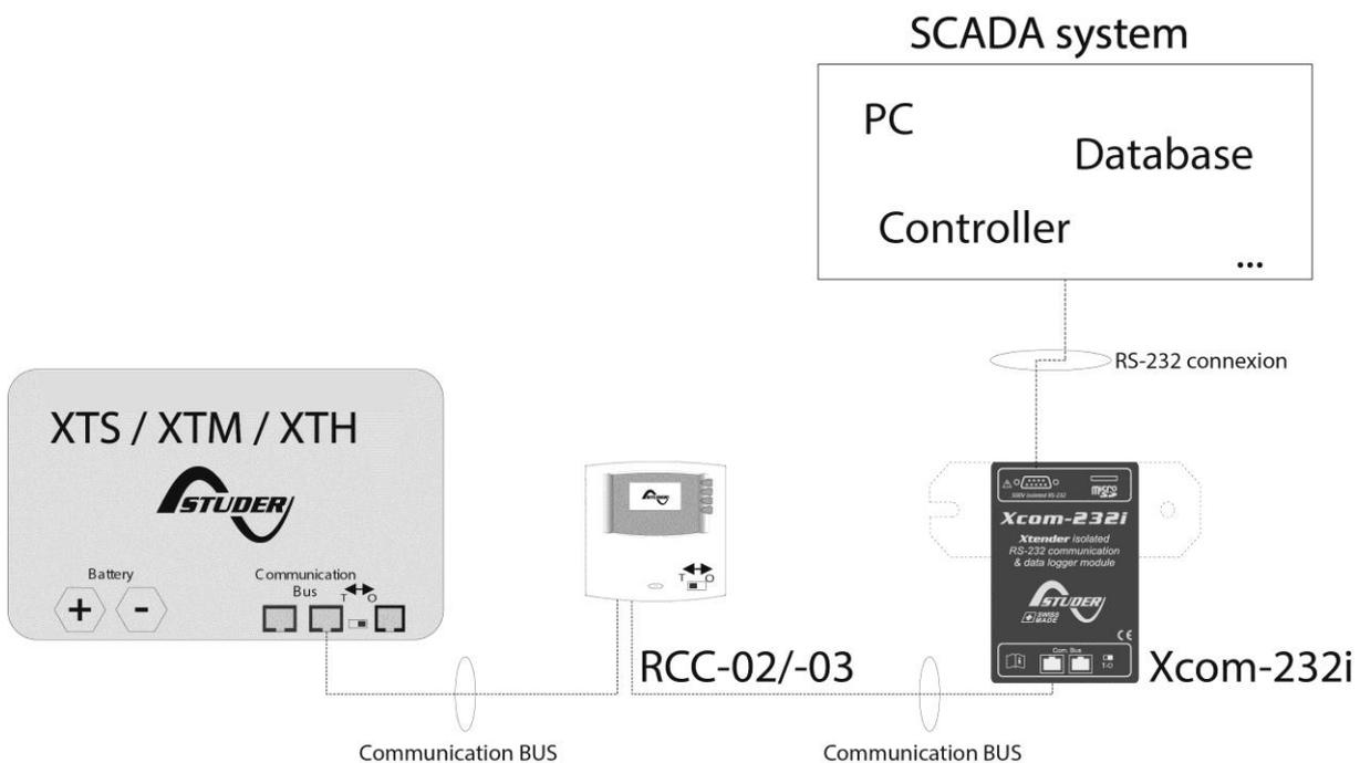
Figure 3.2: Connection schematics of the Xcom-232i (Example 2)
