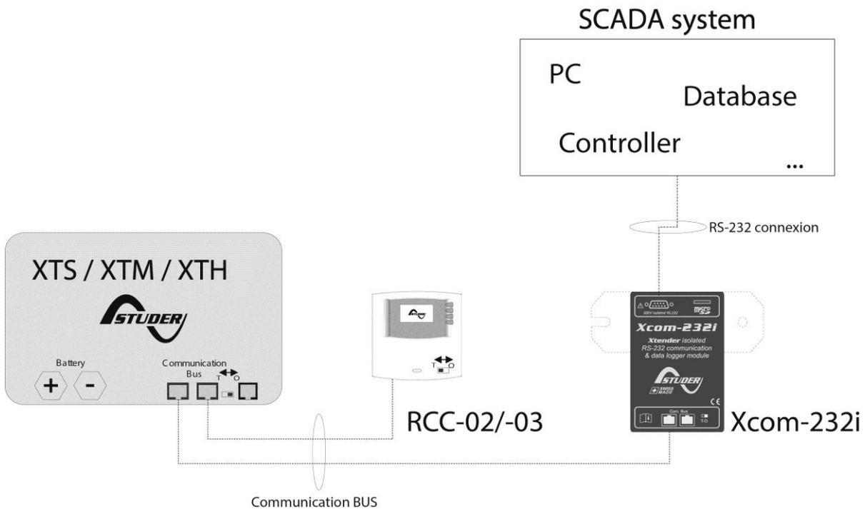
Figure 3.1: Connection schematics of the Xcom-232i (Example 1)
