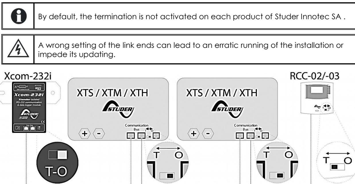
Figure 3.3: Online communication bus of an Xtender system
