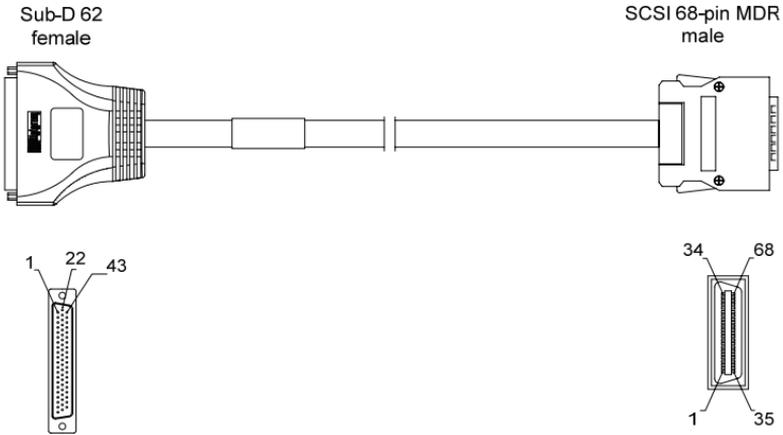
If you dispose of a PCX1221<sup>HR</sup> or PCX1222<sup>HR</sup> cable, this adapter allows its use with the PCX PCI EXPRESS™ multichannel boards.
