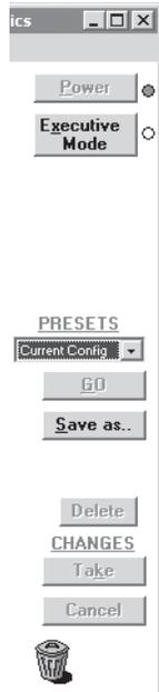
**Power** — Unavailable for TPX switchers, because the switcher power cannot be controlled via software.
