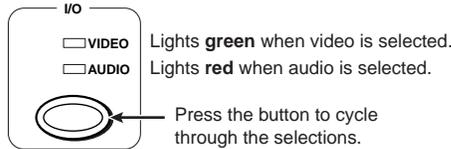
2. Press and release the desired input button.
