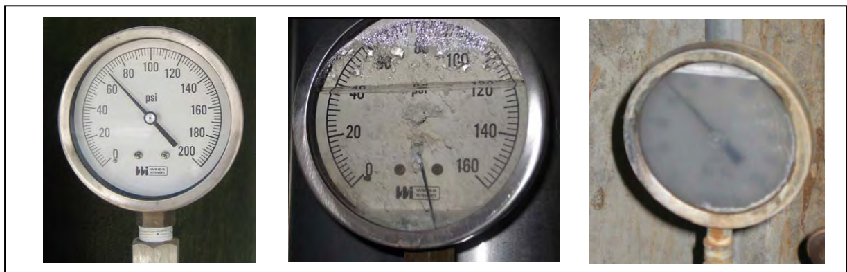
Figure 14 : Examples of a Clean Gauge and Two Obstructed Gauges
