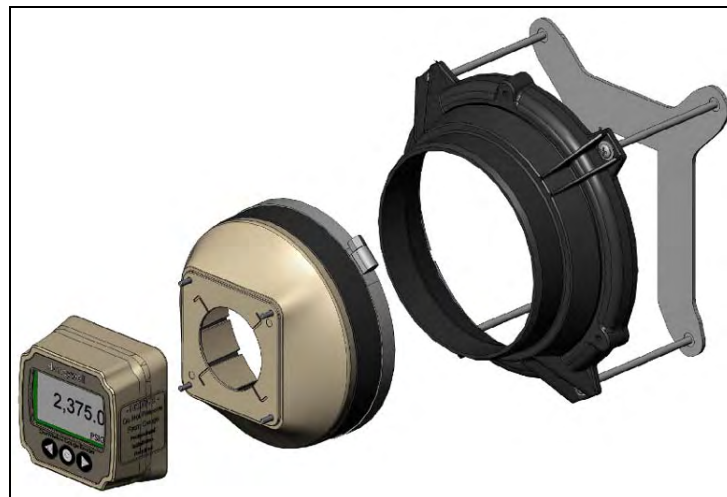
Figure 18 : Installation of a Process Gauge
