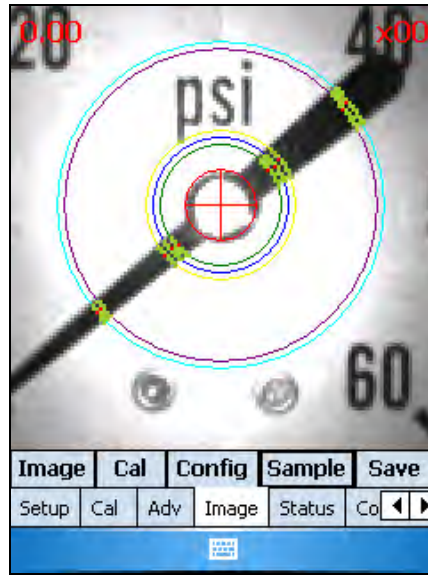
Figure 63 : Green and Red Pixels Superimposed on Image
