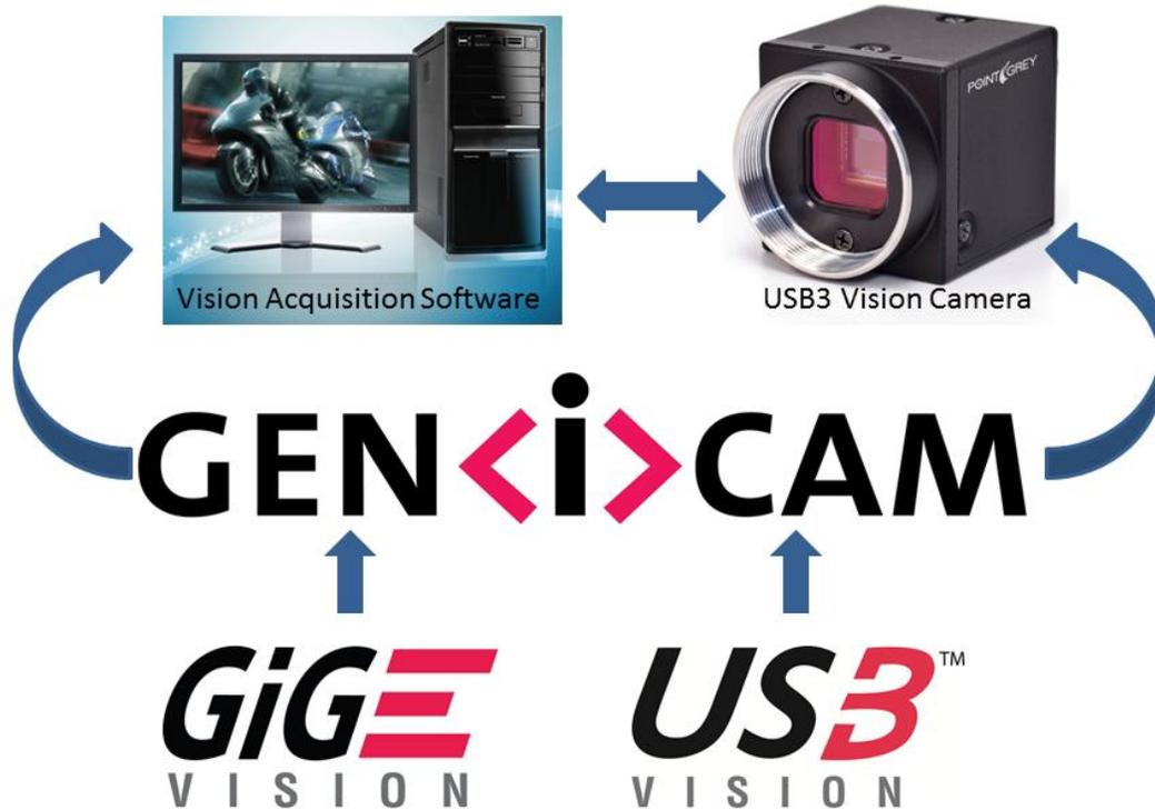
USB3 Vision is a communication interface for vision applications based on the USB 3.0 technology. All cameras supporting USB3 Vision interact the same way with software also supporting USB3 Vision.
