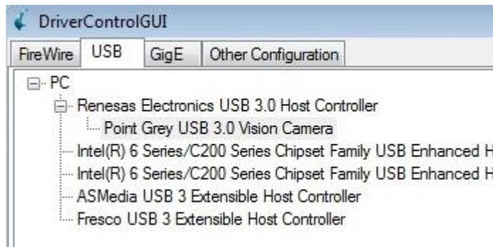
The camera and card are listed as two separate devices.
