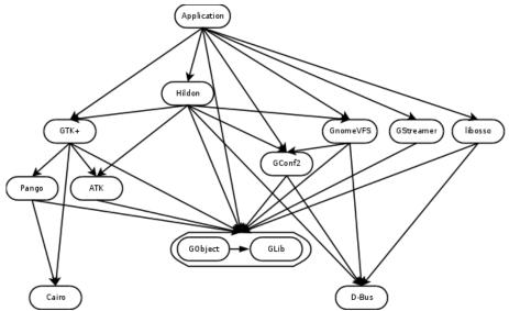
The figure above illustrates the most crucial components and their dependencies that the maemo application developer must deal with. These components are explained in more detail in the next chapters.
