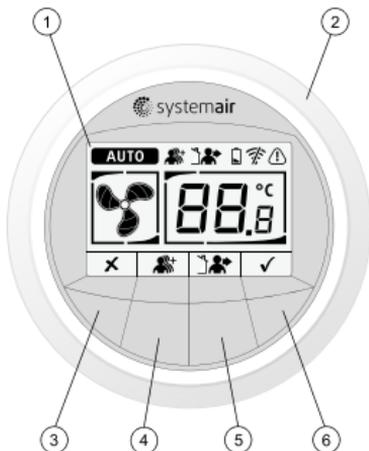
Press the conform button (6) to change fan or temperature settings, then the setting can be changed by turning the dial. When the desired value is shown, press the confirm button (6) to accept the value. Press the cancel button (3) to back out to the starting point (no square active) at any time. If there is no activity for 30 seconds it will automatically back out to the starting point.
