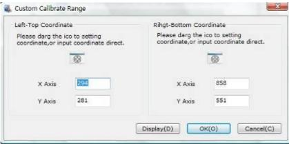
4 points calibration: calibrate by 4 points, for SAW and Infrared touchscreens. 9 points calibration: calibrate by 9 points, for 4W, 5W and capacitive touchscreen. 25 points calibration: calibrate by 25 points, for 4W, 5W and capacitive touchscreen. Select 4 points, 9 points, 25 points or custom and click calibrate to start calibration.
