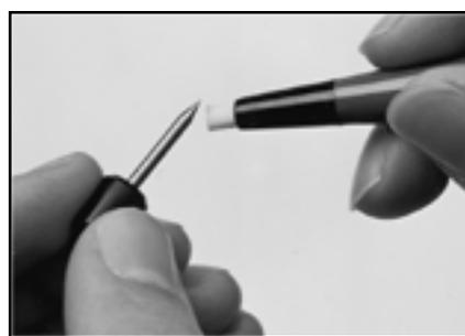
You should remove the **electrodes** and clean them with the fiber glass brush only when error codes 02 or 03 are shown. Do **NOT** clean the electrodes with a cotton swab dipped in alcohol. For instructions as to how you remove and reinsert the electrodes see the section on electrode maintenance on p. 21. Once you have them remounted, you should run the electrode cleaning program (Program 100, see below) 2-3 times.
