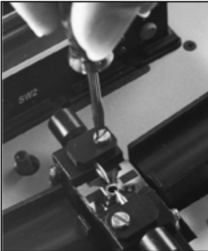
When the error code 04 is displayed, 1000 splices have been executed on the splicer. This is a signal to you that you may want to change the electrodes. You certainly want to replace them every 2000 splices. To get rid of the error message you must reset the splicer counter (see p. 16), and if you are replacing the electrodes you should be resetting the counter anyway.
