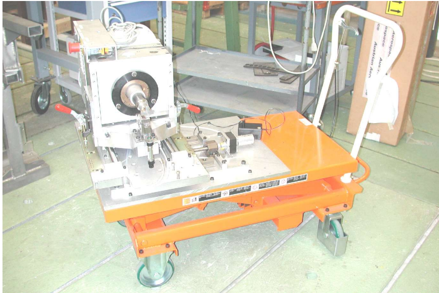
Figure 3 : Welding machine on its support frame
