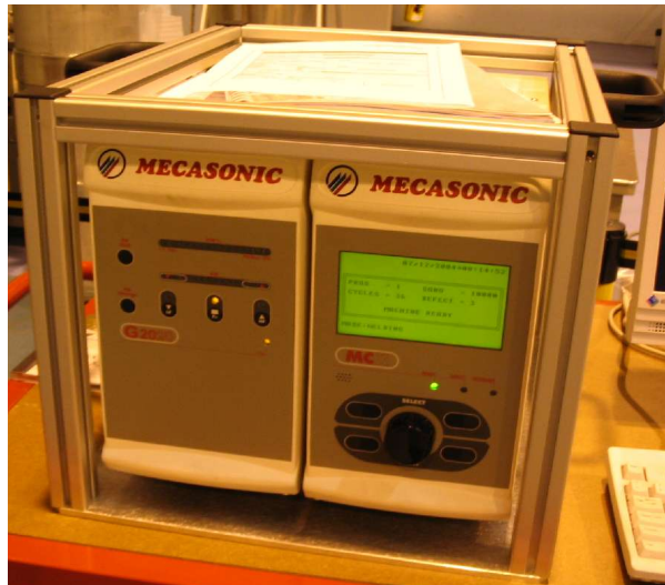
Figure 4 : Front view of the ultrasound generator (left) and the control box (right)
