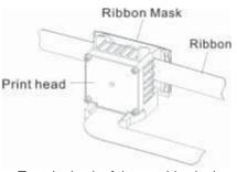
Turn the knob of the cartridge in the direction of the arrow to tighten the ribbon.
