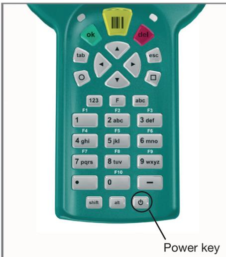
Fig.19 Switching on the power
