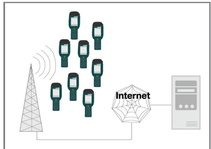
Fig.2 Network over GSM/GPRS
