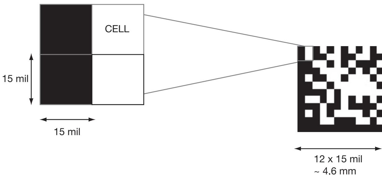
Figure: DataMatrix (15 mil) ID symbology cell and code size (not in actual size)
