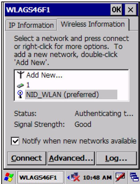
Fig: Detected networks in range. NID\_WLAN is being connected. Authorisation process in progress.
