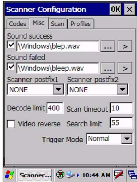
Fig.68 Misc -tab in the Scanned Configuration program
