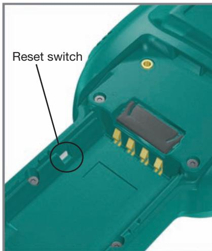
Fig.30 Reset switch of PL3000
