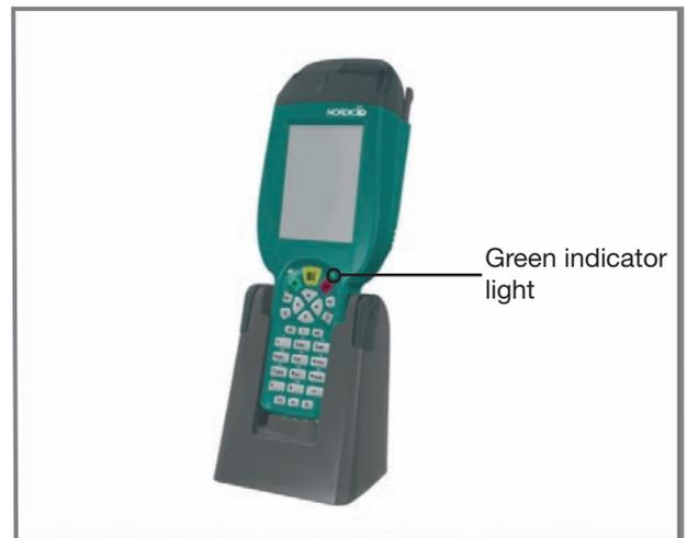
Fig.17 Green indicator light shows that battery is full
