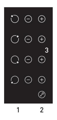
CONTROL PANEL 1. ON/OFF control 2.Keylock control 3. Power regulating controls ۲
