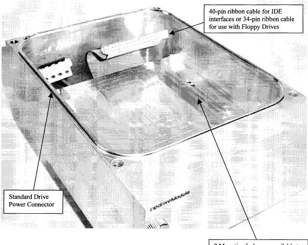
8 Mounting holes are available to secure the drive into the frame.
