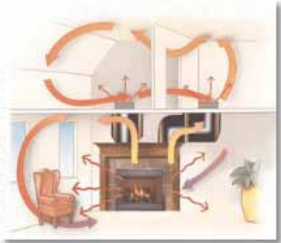
Illustration shows natural convection and Power Heat Duct Kits
