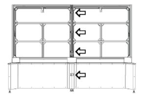
6. Tether the entire floor mount assembly to a wall or floor for added safety.
