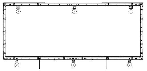
2. Secure 3 brackets to the wall below the LCD panels using 4 screws in the corner holes only. The 3 holes that run vertically down the center of the bracket are used to engage the threaded rod on the bottom frame which allows for adjustment.
