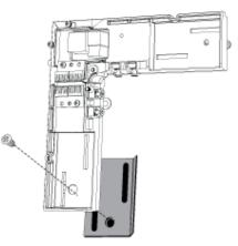
f. After removing the metal bracket, reinsert the corner piece into the master controller sensor board and reassemble the master controller by following these steps in reverse order.
