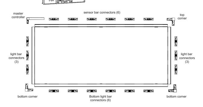
1. Starting at one side, begin installing connector bars to the front side of the interactive subframe. Fasten with 2 screws each.
