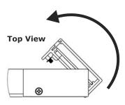
2. Once the sensor bar is installed, adjust the connector bar slightly to center its captive screws with the slots on the bottom of the sensor bar. Loosely tighten screws at this point to allow for later adjustments once all the sensor bars are installed.
