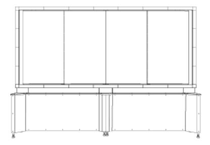
The floor mount is an alternative method for mounting the FHD551-XG panels of a Multi-Touch Video Wall with the Interactivity kit. It is shipped as two separate halves that get fastened together. The LCD flat panels and the interactive frame gets mounted directly to the floor mount.
