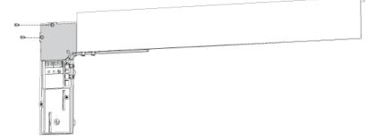
c. On the back of the master controller, remove the 2 screws from the plastic cover around the USB port, ethernet port, and power connection and the 1 screw beside the ports.
