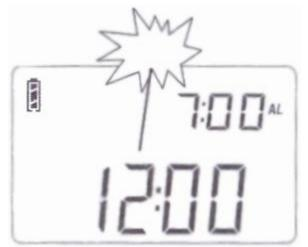
Quick press the [TIME] button again, to confirm the adjustment and setup.
