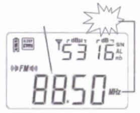
[NOTE]: When PL-360 radio is working in auto scan tuning mode and has the stations is captured, quick press the [MEM] button will save this station in the memory.
