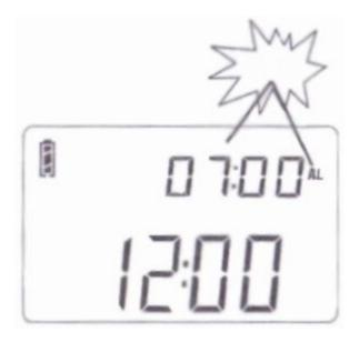
Implement the above steps to setup the auto power on timer, then followed quick press the [ALARM] button again to adjust the auto power off timer after the PL-360 radio auto power on (from 1 to 90 minutes).
