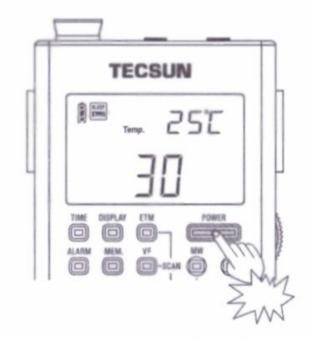
[NOTE]: If can not power on the PL-360 radio, please check the battery installation, battery level, or if the PL-360 radio was locked.
