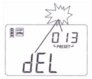
Press the [DEL.] button and hold don't release until has the "DEL" and address number flash on the LCD, followed quick press the [DEL.] button again, will delete this preset station.
