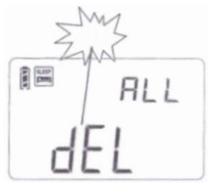
Quick press the [DEL.] button again, will delete the all current band preset stations in the memory.
