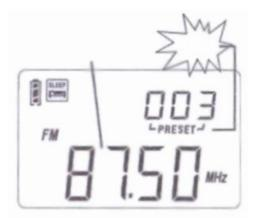
When the ATS tuning finished, the PL-360 radio will auto enter the address status, please turn the [TUNING] knob to listen the stations preset by ATS tuning.
