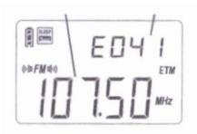
[NOTE]: EMT tuning mode support 100 stations on FM band, 100 stations on MW band, 100 stations on LW band, and 250 stations on SW band.
