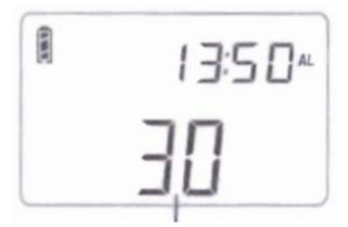
Quick press the [ALARM] button again, to confirm the adjustment and setup.
