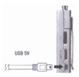
There is a mini-USB interface designed on the PL-360 radio, use the USB 5V power supply to smart charge the Ni-MH rechargeable battery is available. When the PL-360
