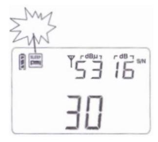
Quick turn [TUNING] knob, select the auto power off time cycle from 1 to 120 minutes.
