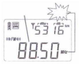
When the PL-360 radio captures the station you would like to preset, quick press the [MEM.] button will auto preset this station in memory. Repeat the above steps to preset next station.
