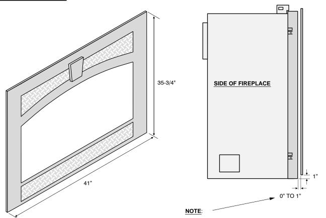
This face has an adjustable bracket that allows for different facing depths to be tucked under the face.
