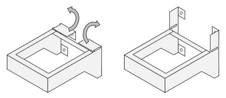
2 Attach the aromatherapy bracket to the back of the face following the directions below.
