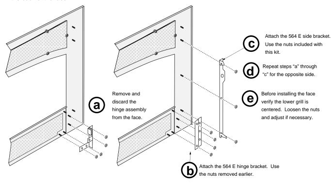
Pull the electric fireplace out of the mantel (or built-in location). Attach the cove cover and face following the directions below. Slide the fireplace back into place to complete the installation.
