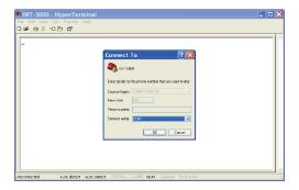
After connection, user can see the above window settings. Before setting, please make sure that the instrument ports have been set, and the terminal should be assigned to the correct COM Port of the instrument. Otherwise, the terminal would not be able to carry out this function.
