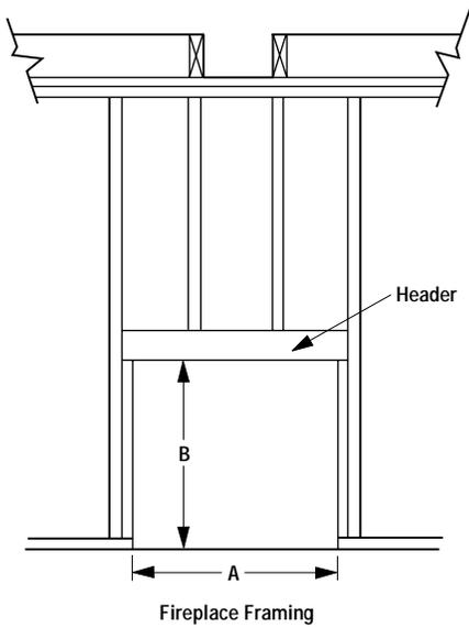
Note: When Framing With 6" Studs Header Must Be 17" (432mm) Higher. Use Security's OR15 Offset/Return Elbow To Recess The Chimney Back 2 1/2" (64mm). Maintain Required Clearance To Chimney At All Times.
