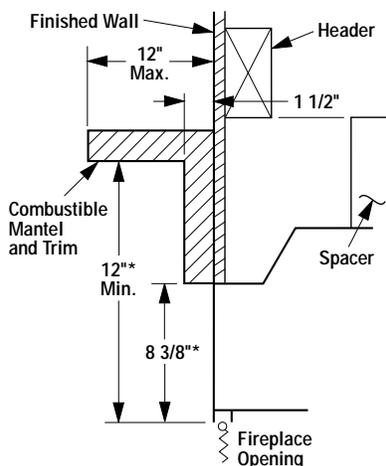
**\*Both Of These Dimensions Must Be At Least 18" When An Unvented Gas Log Set Rated At 26,000 BTU Or Higher Is Used. (Maximum 40,000 BTU)**
