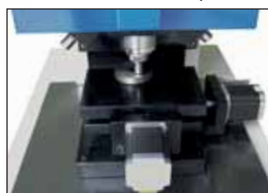
② Motorized turret at 5 - 3 - 2 steps self switch indenter - objectives
