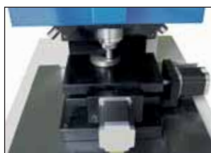
③ Motorized X Y table for series of Vickers test and auto recognize zero point
