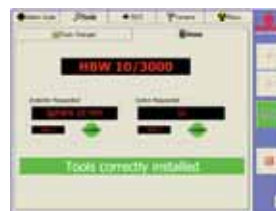
Automatic check-up correct objective and indenter installed on
