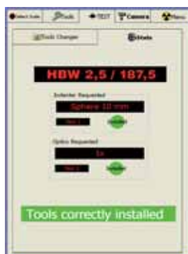
Automatic check-up correct objective and indenter installed on
