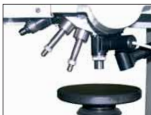
② Motorized turret at 5 - 3 - 2 steps self switch indenter – objectives
