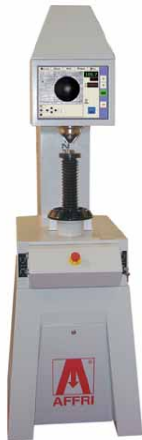
② Motorized turret at 5 - 3 - 2 steps self switch indenter – objectives
