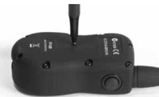
For example, if mode 5 is desired, adjust the Intensity Dial to Level 5. Once the Mode Button has been depressed, the Transmitter Indicator Light will be solid and, once the mode button is released, the Transmitter Indicator Light will flash 5 times.
