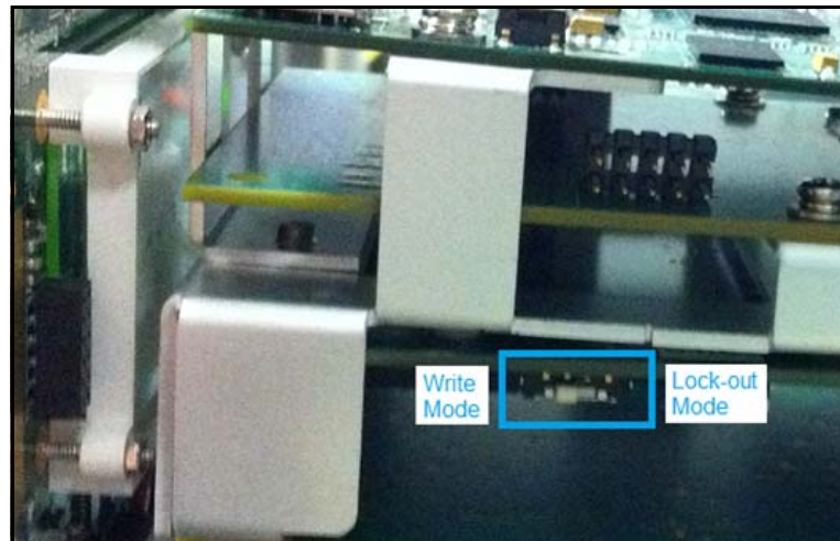
Figure 35: HART Circuit Write Mode Switch. With the Write Mode switch pushed toward the Display board (as shown), the HART circuit is in write access mode.
