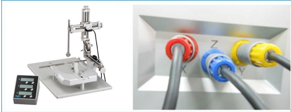
Fig.2 Connection Diagram of each X-, Y- and Z-Axis Sensor to Digital Display Module
