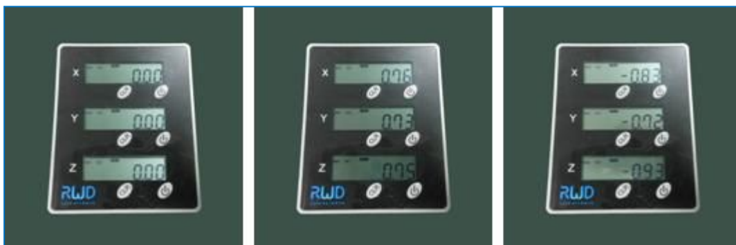
Fig.3 Diagram for Zeroing and Real-time Displaying of X-, Y- and Z-Axis Readout respectively
