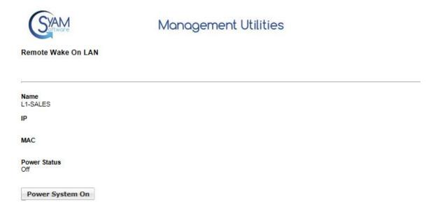
Click the Power System On button. The system power status will be reported as On when the machine responds to ping, or when the System Client is initialized. If the system is still off after five minutes, it may be unavailable on the network or not properly configured for Wake on LAN.
