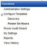
The Power On Hours Template specifies the hours that a group of machines should be powered on. Use the default template or create your own. The easiest way may be to copy the default template and then make any desired changes.
