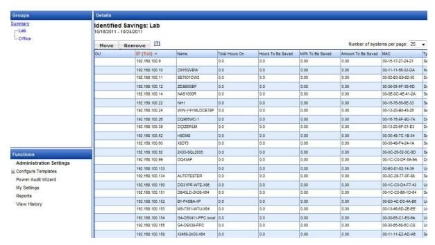
New groups and subgroups can be created, and systems can be moved from one group to another. For example, discovery of systems across an IP range may create a group with a mix of desktops and servers. Servers could be moved into a separate group, with a different Power On Hours template used for that group. Settings can also be changed within a group by highlighting a row (or rows) and using the right-click menu to change system classification, wattages, or the Power On Hours template.
