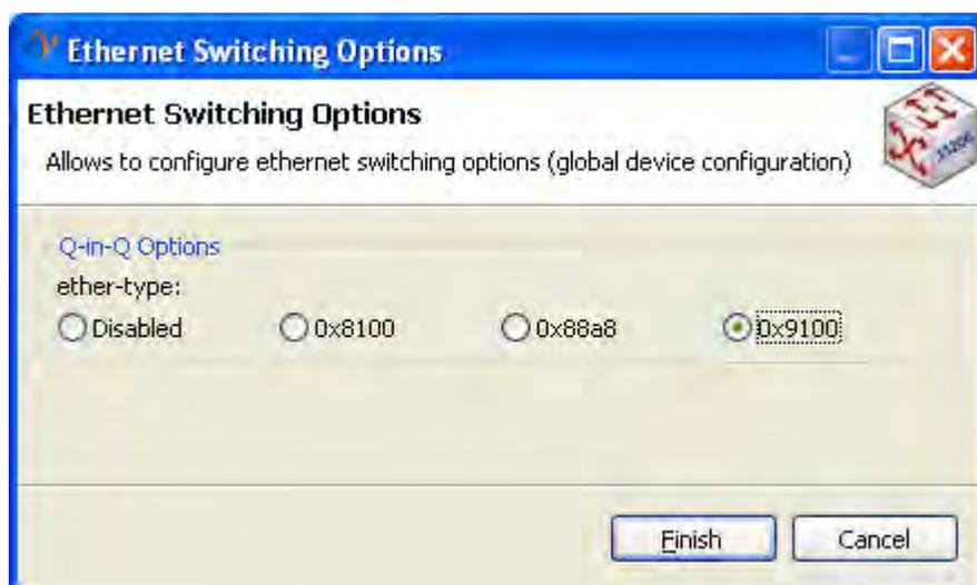
Fig. 2-42: Ethernet Switching Options
