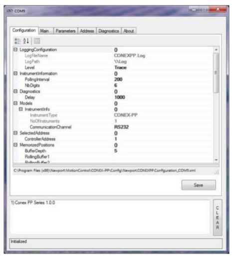
The polling interval defines the number of milliseconds between each time the Controller GUI polls the CONEX-PP series for the latest information. The user may change the polling interval by entering a value. Diagnostics Delay defines the time delay in milliseconds between each command sent from a text file.
