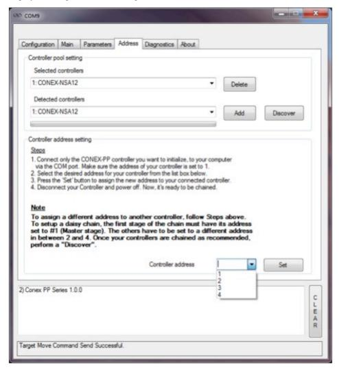
Now disconnect this controller from your PC and connect the next one. Select a new, unallocated address and press the "Set" button again (proceed the same way with all other controllers).
