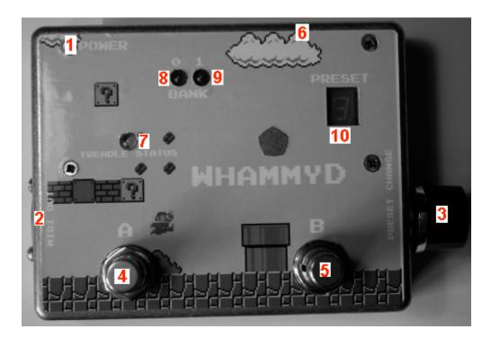
**1 – Power connector** (You may use any power adaptor with voltage 9-12 V, 100 mA and more, AC/AC or AC/DC).
