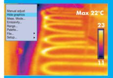
**LOCATE AND ANALYZE PROBLEMS FAST** Analyze problems and share results with your colleagues in the field. Movable crosshairs allow you to measure and analyze the temperature at a single point. Find the hottest spot in a defined area, highlight areas of concern with color or sound alarms. The ThermaCAM B4 has all the analysis tools you need to make instant building decisions in the field.
