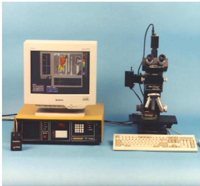
Figure #2 A typical ThermoMap system implementation is shown above with a Temptronic ThermoChuck/Socket temperature controlled platform, microscope with camera attached, IC device with power supply, Pentium-based personal computer (PC) and ThermoMap software.
