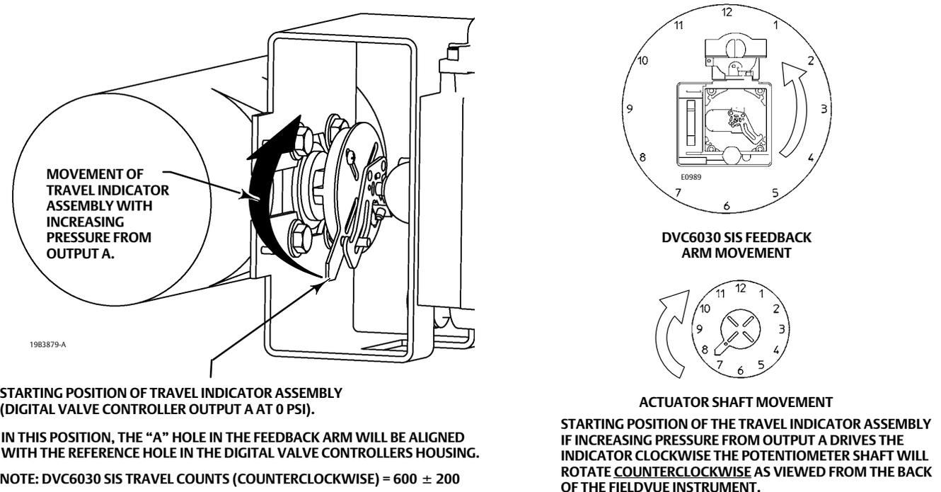
7. Position the digital valve controller so that the pin on the travel indicator, engages the slot in the feedback arm and that the bias spring loads the pin as shown in figure 10. Attach the digital valve controller to the actuator or positioner plate.
