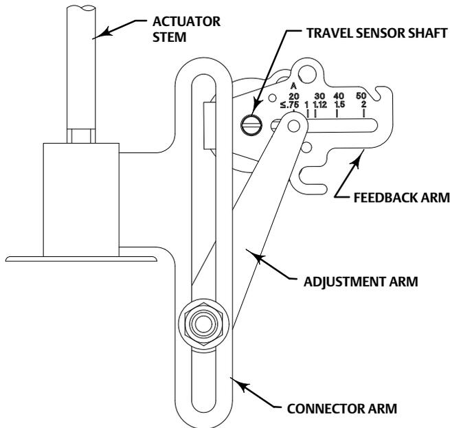
Figure 24. Feedback Connection for Typical Long-Stroke Sliding-Stem Actuator (4 to 24-Inches Travel)
