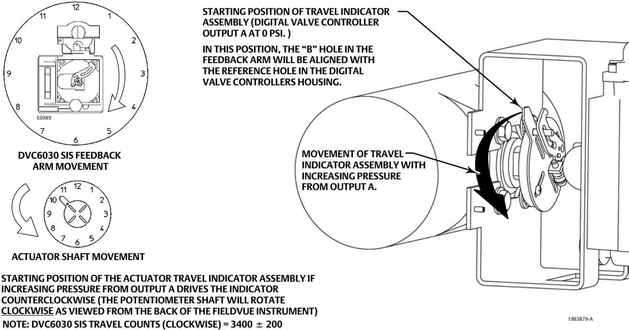
Figure 9. Explanation of FIELDVUE DVC6030 SIS Travel Indicator Starting Position and Movement if Counterclockwise Orientation is Selected for “Travel Sensor Motion” in ValveLink Software or the Field Communicator
