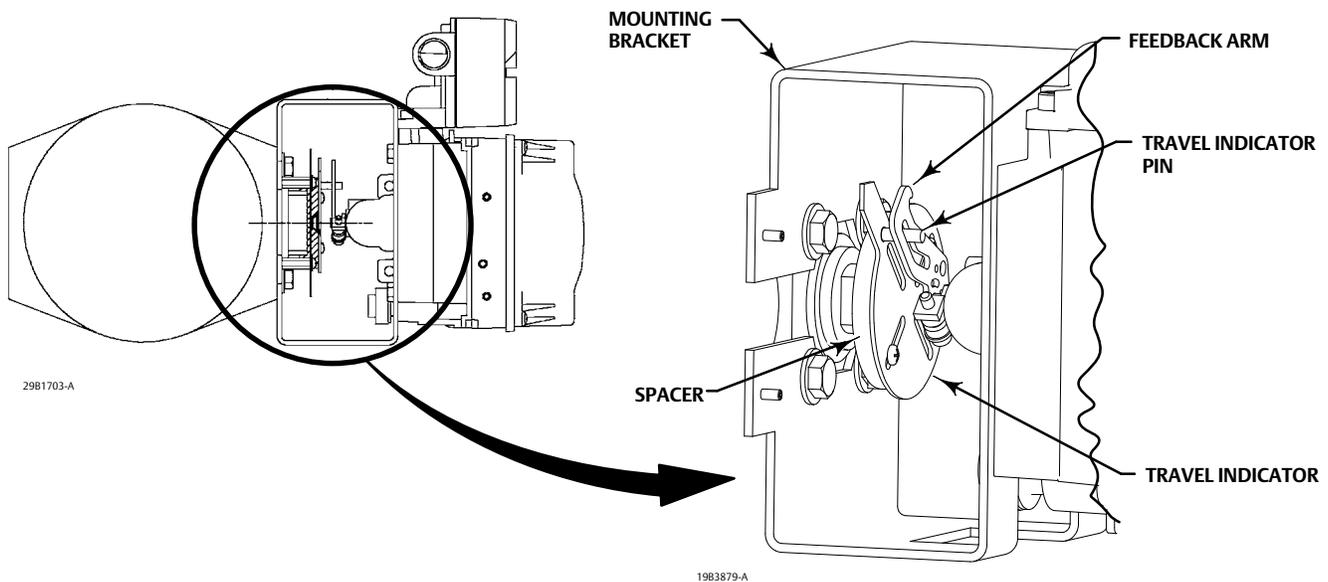
4. If required, attach the spacer to the actuator shaft.
