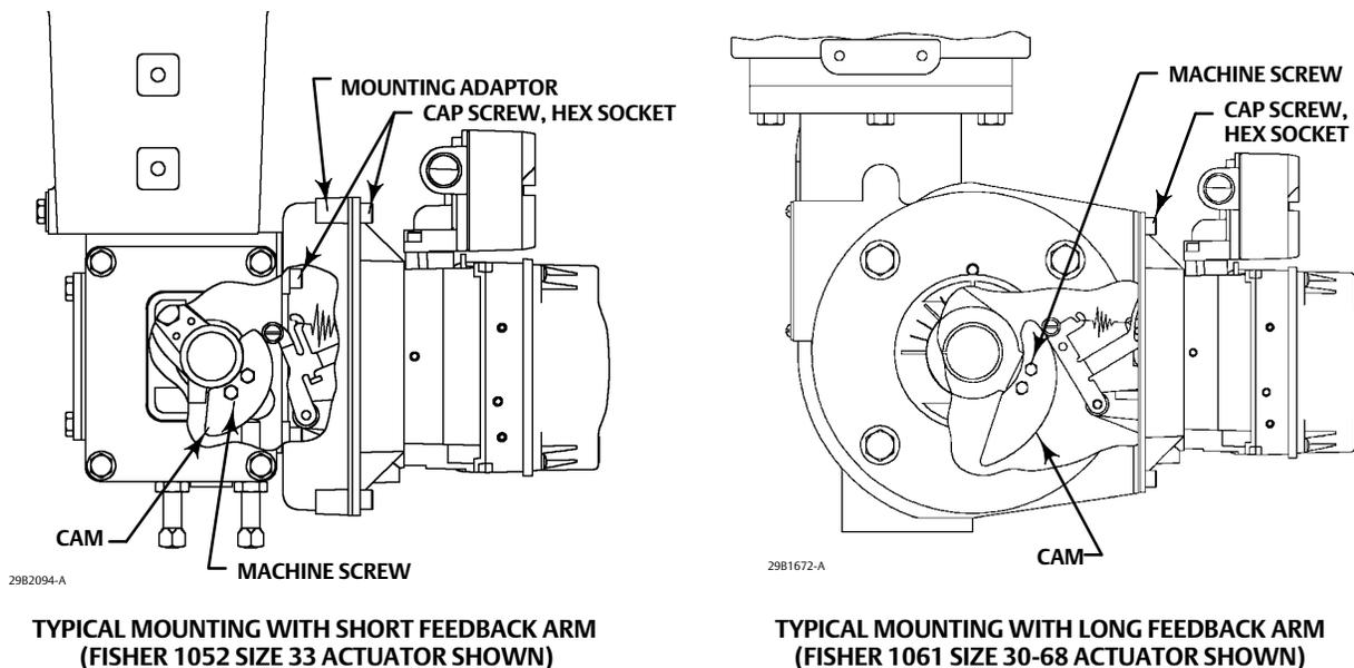
Refer to figure 5 for parts locations. Refer to the following guidelines when mounting on rotary actuators:
