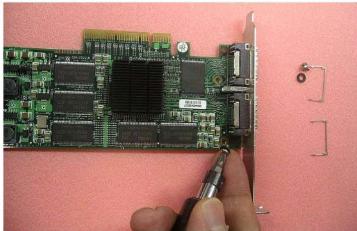
Figure 13: Attach Bracket onto Card using Screws
