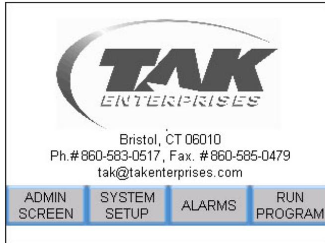
When the system starts up this will be the first screen showing. From this screen you will be able to access Administration functions, System running functions, System alarm information and the Program running section. To access any of the screens from here just touch the appropriate screen button. If the screen you are trying to access is password protected you will be shown a keypad to enter the code. **The Supervisory password is 3333.**
