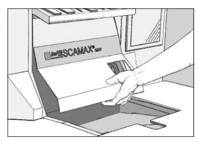
Next, the cover plate over the feed mechanism needs to be removed. To this end, loosen the two recessed-head screws.
