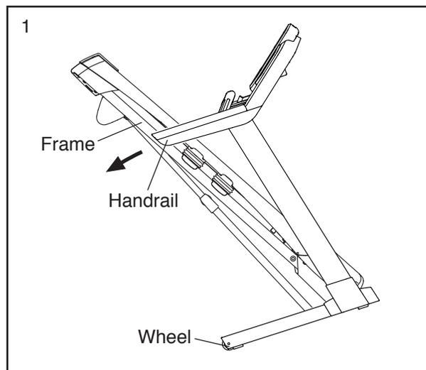
2. Pull back on the handrail until the treadmill will roll on the wheels, and carefully move it to the desired location. **CAUTION:** Do not move the treadmill without tipping it back, do not pull on the frame, and do not move the treadmill over an uneven surface.
