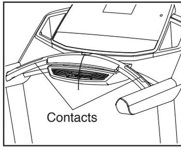
To measure your heart rate, **stand on the foot rails** and hold the pulse bar with your palms on the metal contacts; **avoid moving your hands**. When your pulse is detected, several dashes will appear and then your heart rate will be shown. **For the most accurate heart rate reading, continue to hold the contacts for about 15 seconds.**
