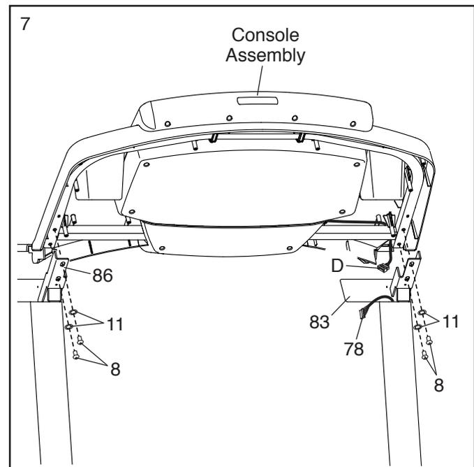
8. Attach the console assembly to the Handrails (83, 86) with four #10 x 3/4" Screws (7) and four #10 Star Washers (14) as shown. **Start all four Screws, and then tighten them.**
