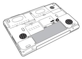
Removing the battery pack-1
