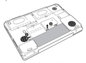
Removing the battery pack-2
