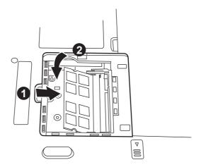
Installing a module
