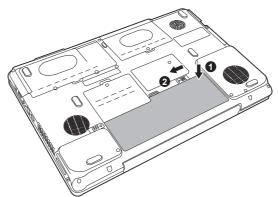
Installing the battery pack
