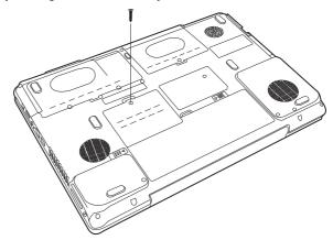
Removing the memory module socket cover
