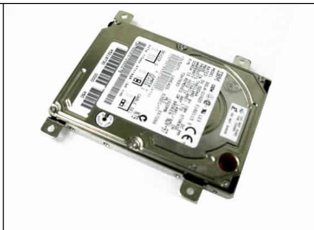
**Fig. 2-15b** Fix HDD to the bracket
