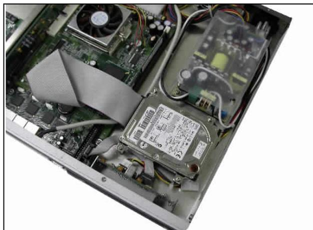
**Fig. 2-18** Drive all four screws back
