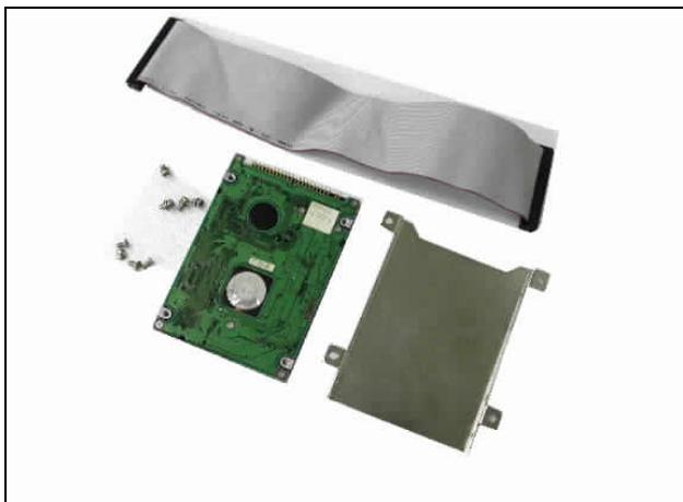
**Fig. 2-15a** A 2.5" HDD and the HDD bracket
