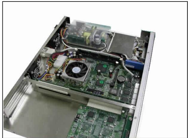
**Fig. 2-12** Completion of DOM power connection
