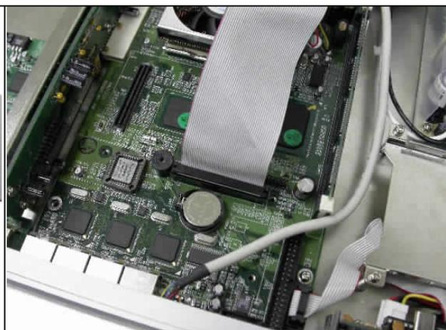
**Fig. 2-17** Connect IDE cable to PPAP-250
