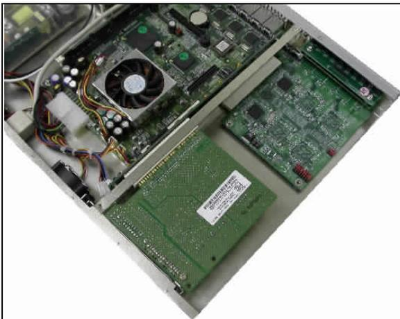
**Fig. 2-21** Push the PCI add-on card into the PCI slot
