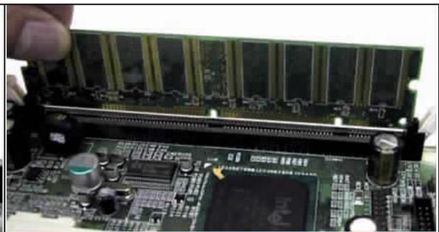
**Fig. 2-7** Install DIMM
