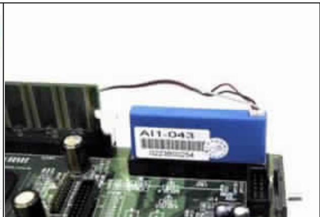
**Fig. 2-9** Insert DOM into IDE interface
