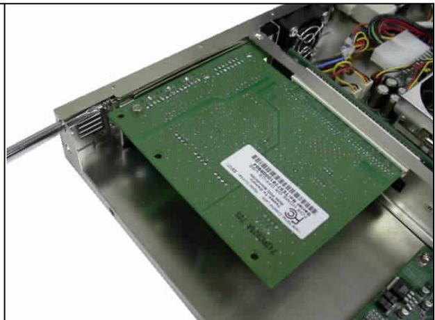
**Fig. 2-22** Fasten the screw back to the side
