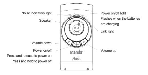
Power on/off Press and release to power on Press and hold to power off Microphone e mamia Hush
