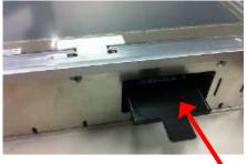
Step 4 Close the cover of CFast<sup>™</sup> card slot and fix it. Installation completes.
