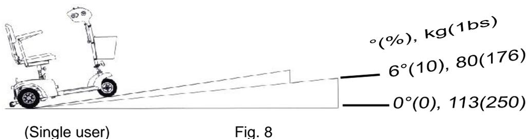
Angles and weights shown here for this scooter indicate the safe working angles for the user and equipment. Any scooter used outside these parameters may be unsafe and or cause future problems with the electrical systems
