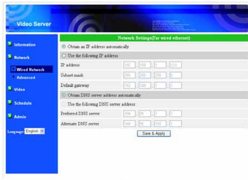
Figure 3-7 Network settings page for DHCP function
