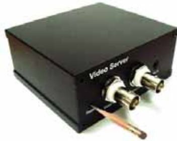
Fig. 3-27, stick 5 sec to the factory default settings.
