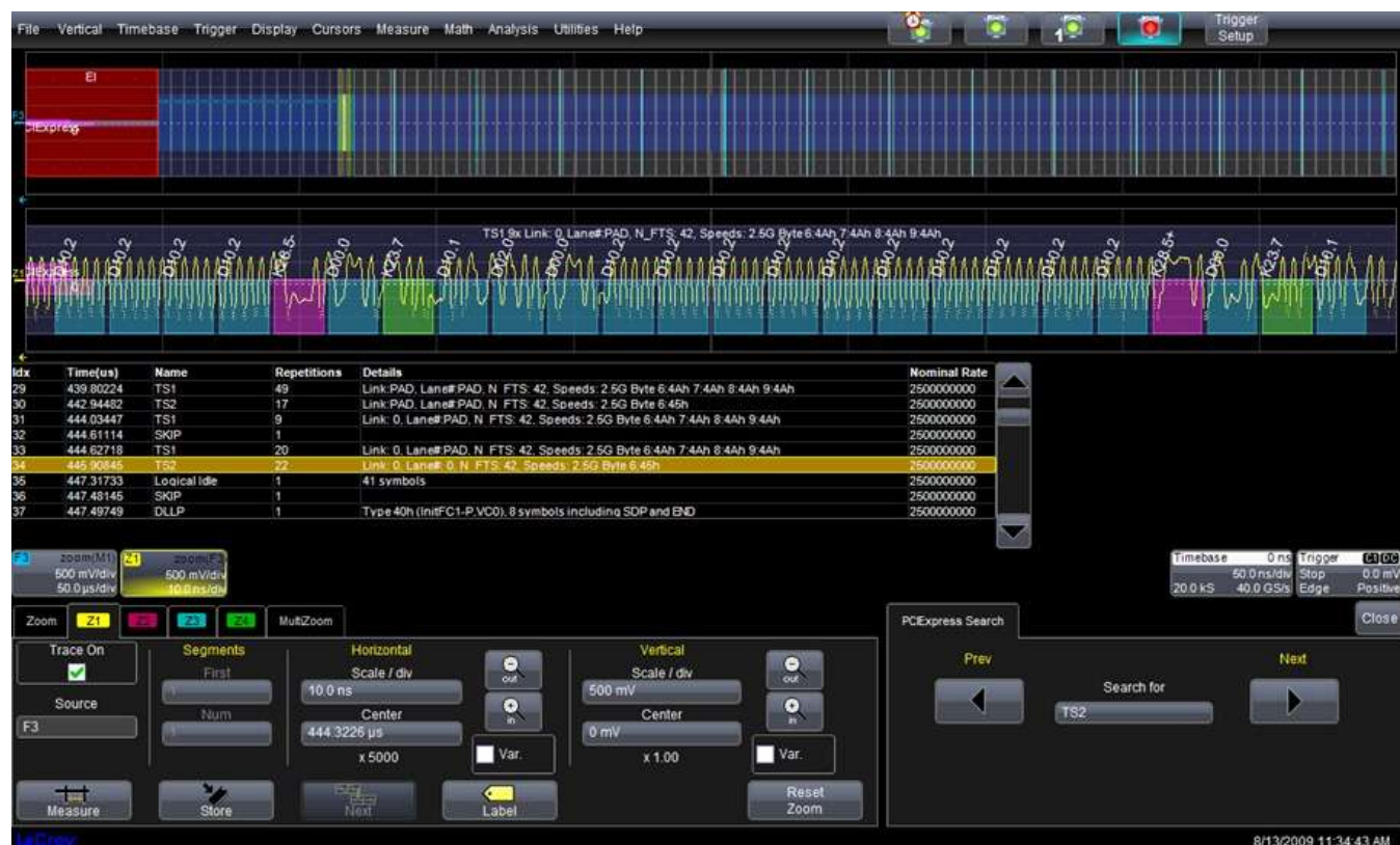
Figure 3-7. Zoomed in on Z1, showing the 8b/10b decode of a TS1 sequence.
