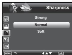
**STRONG** Increases contrast on the edge of the picture. Image color noise (grain) may occur in the recording image.
