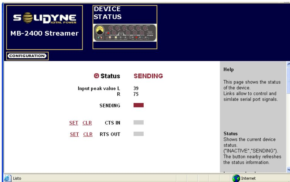
It presents the state of the streamer module MB-2400. The most important parameters are:
