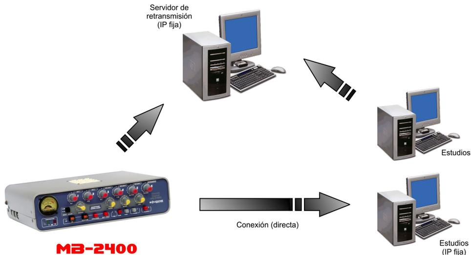
*This scheme is a summary of the ways that you can work when the MB-2400 starts the connection. Note that in case A, both the console and the studios start the connection to a streaming server .*
