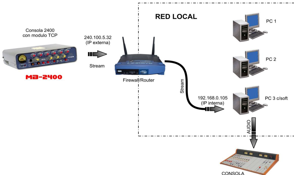
The diagram shows the path to the streaming audio from the console to the PC host for an IP connection.
