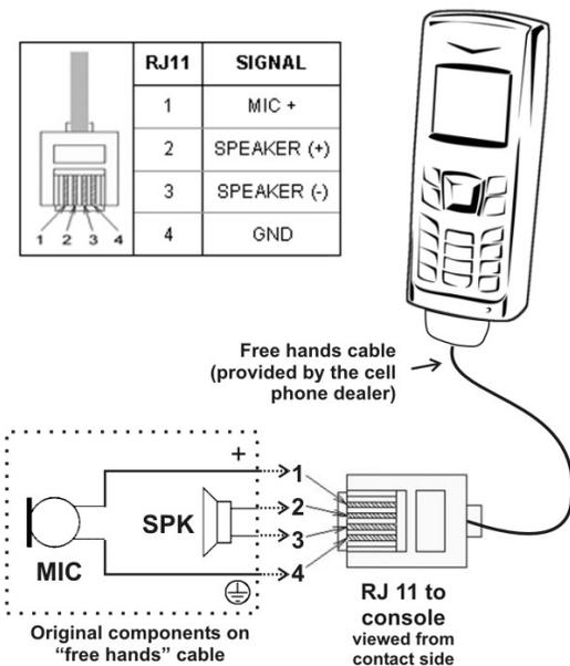
What cell phone transmits through this connector are the audio signals from cell phones. The console sends PGM signal to the cell, which transmits to the radio. The radio sends back to the telephone, which enters through the cell phone to the console and sent to the headphone mix (Studio). Usually, the microphone and speaker phone are disconnected while using the audio connector for hands-free.
