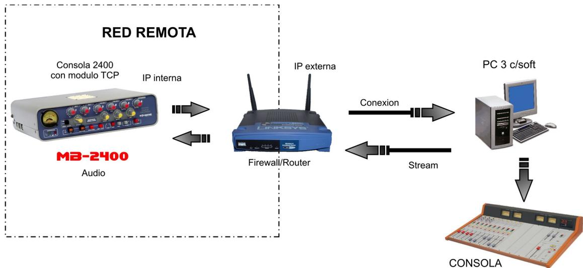
Connection scheme originated in a study destination console connected to a remote local area network.
