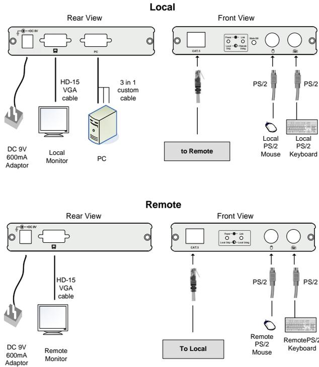
1. Connect PC console port by using standard 3-in-1 cable to Local. (First connects PS/2 mouse, then connects PS/2 keyboard and VGA connector).
