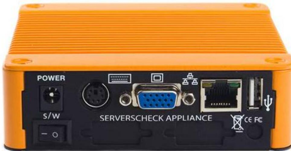
On the back of the appliance you can connect a monitor using a standard VGA cable, a PS2 keyboard and a mouse. If you don't have a PS2 keyboard then you can also use an USB keyboard using the USB port on the front. When connected you will be prompted with a standard windows login screen as shown below.
