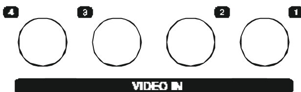
Figure 1.11. Female BNC connectors for camera connection
