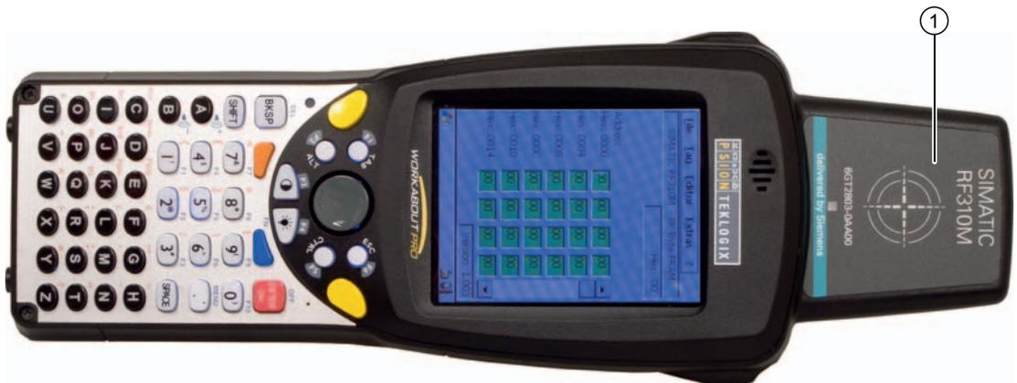
Figure 2-1 Read head with antenna
