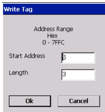
Figure 6-9 Entering the start address and length for the write area
